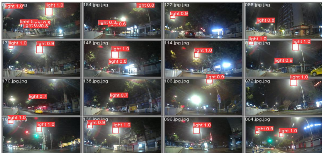
Figure 5: Some streetlight detection results in complex scenarios
